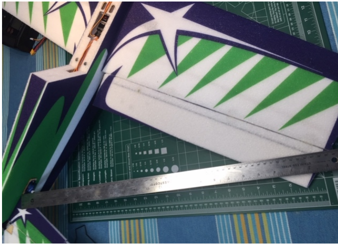
14 Ensure Wing is Perpendicular to Fuselage.
