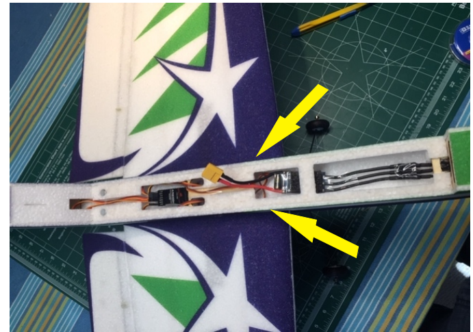
15 Install Servo, Aileron, Control Horn and Servo Linkage to other Wing as in Step 12 Medium CA Wing
