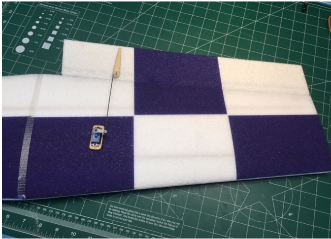
12 Install Servo and Aileron in one side of Wing only. Install Control Horn and Servo Linkage Medium CA Hinges
