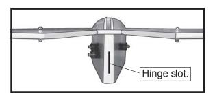
2) Glue the vertical fin in place using as same as techniques used to installing the horizontal fin.
